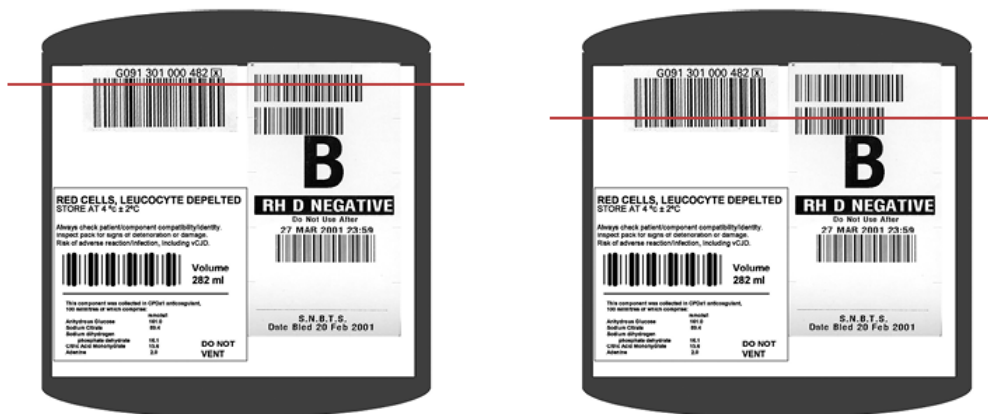
Figure 23.2 Two concatenation processes. On the left the donation identification number (DIN) with nationally defined structure, and on the right the DIN with the ABO/Rh blood group barcode
